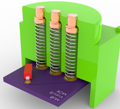
Single block, featuring three independently sprung pins
