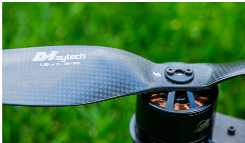
The 18" carbon fiber propellers , capable of providing enough lift to carry the entire hybrid system , with ease
