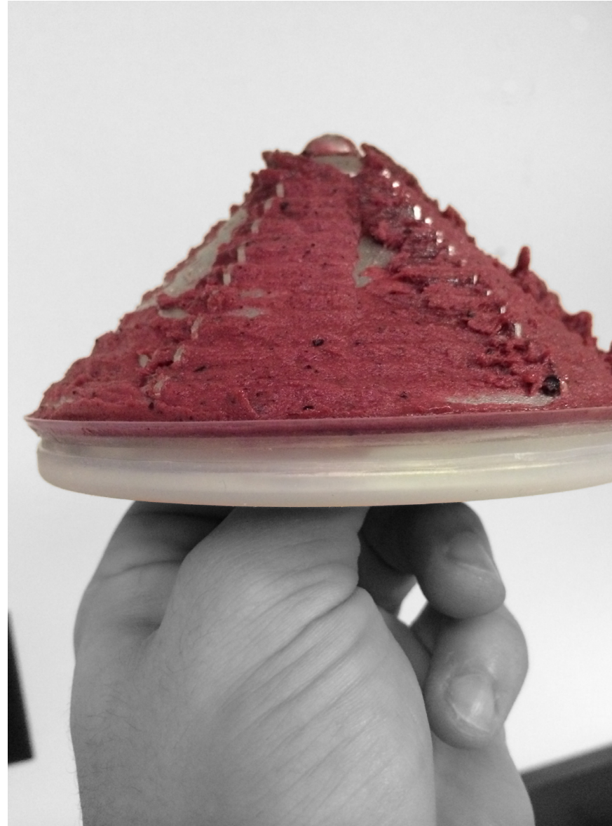
My redesigned cutter head seal solved all problems related to fruit blowby, while decreasing the friction the motor had to overcome to spin the cutter head
